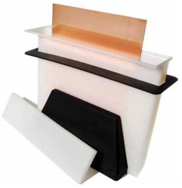
Ferric Chloride Vertical Etching Tank: Z\*Acryl ¼" thick polyethylene structure with a form fitting lid that minimizes evaporation. Holds 4 gallons of ferric chloride and will etch two full 18" x 24" plates. Uses 80% less studio space than a traditional bath-style tray. 8 ½"W x 24 ½"L x 22"H
