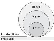
10 34" diameter drum available on Takach floor model etching presses. 7 ½" & 4 ½" diameter drums available on Takach table top etching presses.
