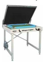
**Direct Screen Exposure Units:** The NuArc First-Light and NuArc Mega-Light units have high output, UV florescent lamps that expose all silkscreen emulsions: direct, capillary & indirect. These affordable direct silkscreen exposure units are enclosed, allowing operation in the darkroom. Weakest UV light source designed for silkscreen use only. Not recommended for Emerald photo litho, or photopolymer plates and films.
