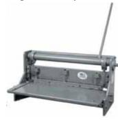
This bench shear features top and bottom blades that are interchangeable.
