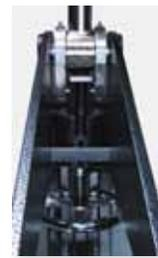
The finest quality hand machined parts ensure ease of operation when applying printing pressure. The pressure system consists of 1” diameter hardened steel pins, custom machined connecting rods, piston and pressure cylinder, and permanently lubricated fiberglide bearings. This system will accommodate stones and plate backers ranging in thickness from 1/2” to 4 1/8”.
