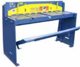
This foot squaring shear includes back and front stops. Made in USA
